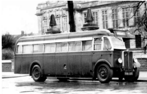
A.E.C. Regal O662 FAX 321 (S131). Originally Green Line Coaches GH 8090 with Hall Lewis C27R body, it passed to L.P.T.B and eventually to the Ministry of War Transport. It was fitted with a new Burlingham body and Gardner 5LW oil engine before entry into service with Red & White in 1944. (Omnibus Society / Roy Marshall)
