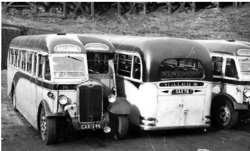
Ralph's 1938 CX13 CAX 344 (70) and the rear end of 1939 CX13 DAX 75 (75). The 1938 model had similar Duple bodywork to the Red & White 1938 SpPV141s in the CAX series.
