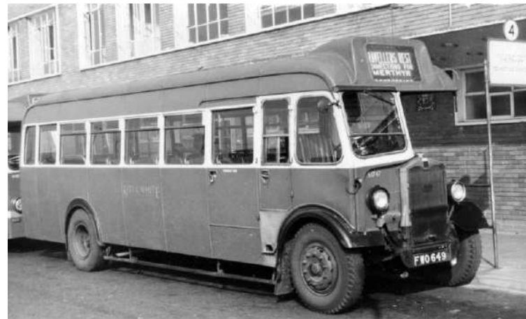
FWO 649(S1747) after receiving the second-hand 1950 B.B.W. body from withdrawn ex-Blue Belle Albion SpPV141 EXF 263 (S3838) in 1957. Note the angular window frames compared to the more rounded frames on the later B.B.W. bodies. This body also differed in having a hinged door at the top of the entrance steps. See the earlier, nearside view of EXF 263 with this body in Section 2.5. (R H G Simpson)
