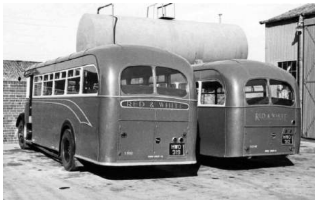
Rear view of two Lydney-bodied Tigers 1950 HWO 319 (S650) and 1949 HWO 312 (S1249) showing the difference in rear end styling and height of the 1950 model.
