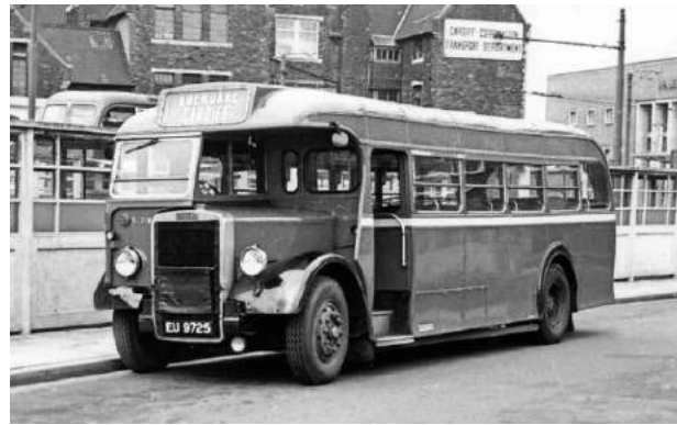
ex-Griffin Lydney-bodied Tiger EU 9725 (S1749) in the later Tilling-style livery. EU9721-26 were the only Lydney-bodied Tigers to be repainted in this livery presumably because of the waistline trim which was not applied to the later vehicles
