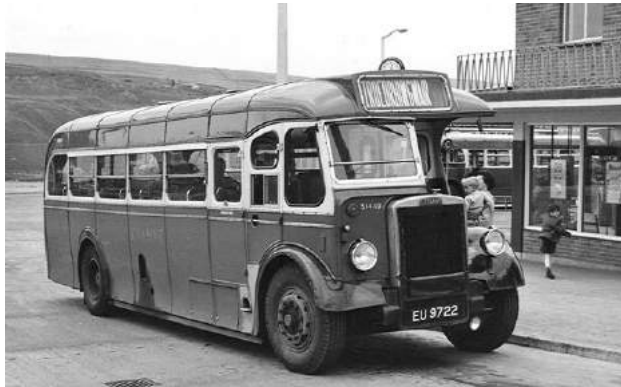
One of the first Lydney-bodied Tigers ex-Griffin EU9722 (S1449). Complaints by Griffin of limited forward vision apparently prompted a change in design of the later 1950 batch which included a higher build line and deeper windscreen.
