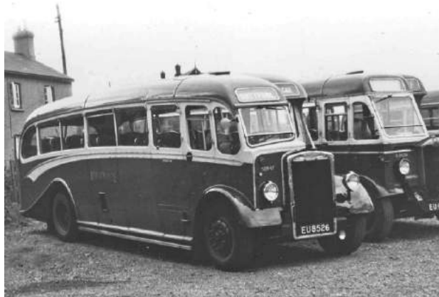
EU 8526 (S2647) after rebodding in 1953 with 1948 Duple C32F body from withdrawn prewar Tiger TS8 BDW 6 (C1137). (R H G Simpson)
