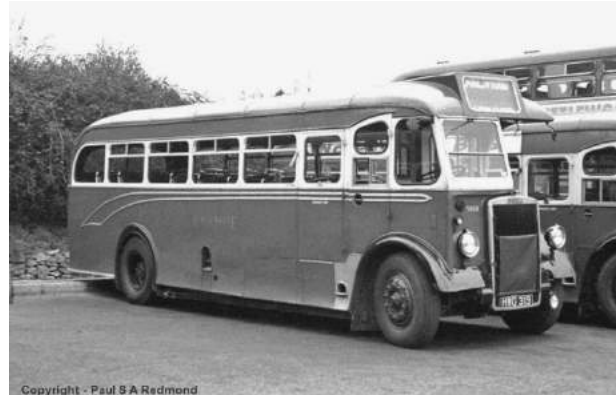
1950 Lydney-bodied Tiger HWO 319 (S650). S150-S650 had detail differences in body styling including a higher build line, deeper windscreen and a Duple-style flash which was absent on the earlier versions. (Paul S A Redmond)
