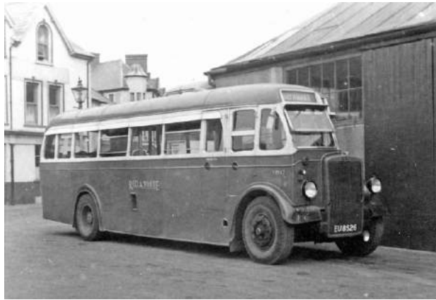
ex-Griffin EU 8526 (S2647) with original Leyland B35R bodywork. (Omnibus Society / D S Giles)
