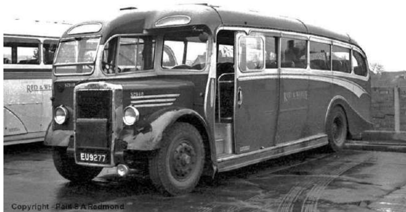
One of the ex-Griffin Duple-bodied Leyland Tigers EU 9277 (S2948) after downgrading. (Paul S A Redmond)
