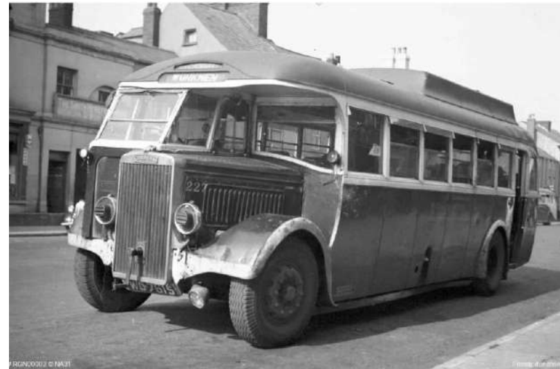
WO 7615 (227) in Monmouth during the war with shielded headlights and white painted mudguards. (NA37)
