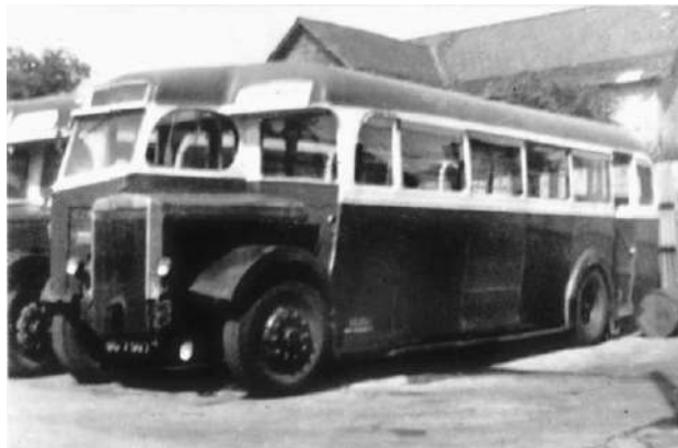
WO 7597 (226) after rebodding with secondhand DP35R E.C.O.C. coachwork from a North Western Road Car vehicle. (Thomas W W Knowles Collection)
