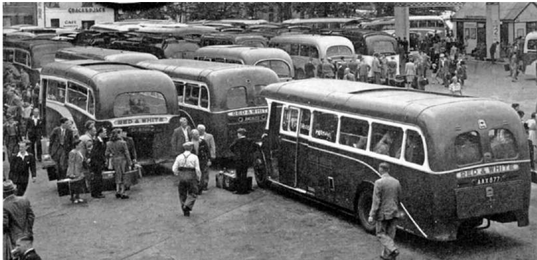
Duple-bodied Albion Valkyries at Cheltenham Coach Station. 1936 Valkyrie SpPW69 AAX 877 (277) foreground and 1936 Valkyrie SpPV141 AWO 620 (307) in front. The coaches have had their roof-mounted luggage carriers removed but still have the rear steps used by the driver to reach the roof. On the left is a 1938-39 Valkyrie CX13. ( Red & White Services 1919-1949 )
