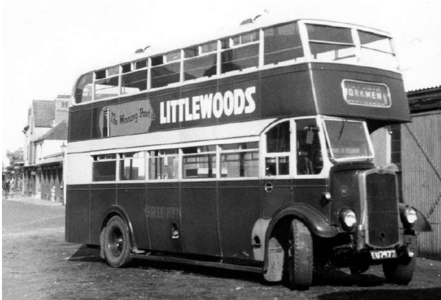
Griffin Bristol K5G EU 7477 (L542) with 1950 Lydney L27/28R body. (Alan B Cross)
