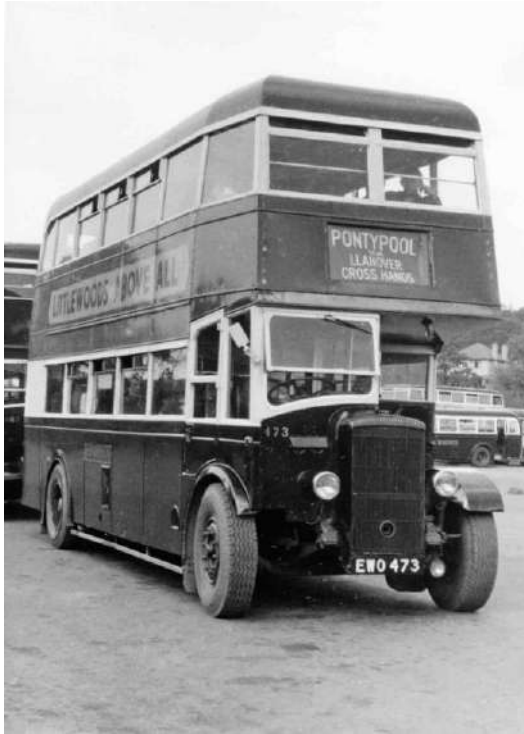
1943 Daimler CWG5 EWO 473 (later H443) with highbridge Massey UH30/26R bodywork. (Alan B Cross)
