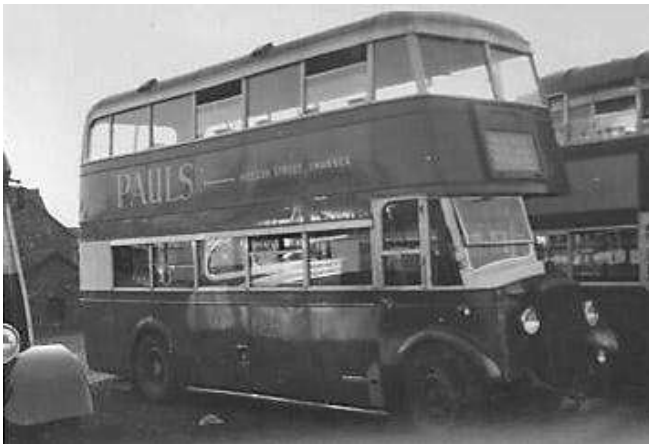
ex-Swan Motors Willowbrook-bodied highbridge Daimler COG5 DWN 2 (840) after transfer to United Welsh.
