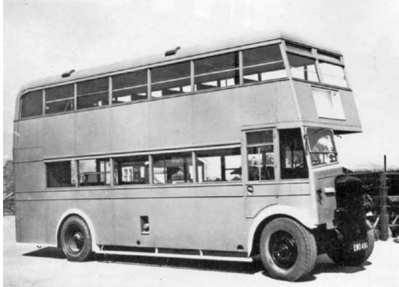
Daimler CWG5 / Brush UL27/28R EWO 486 as delivered to Red & White in 1943 in wartime grey paint and white painted mudguards and platform edging ( Brush Coachworks Ltd )
